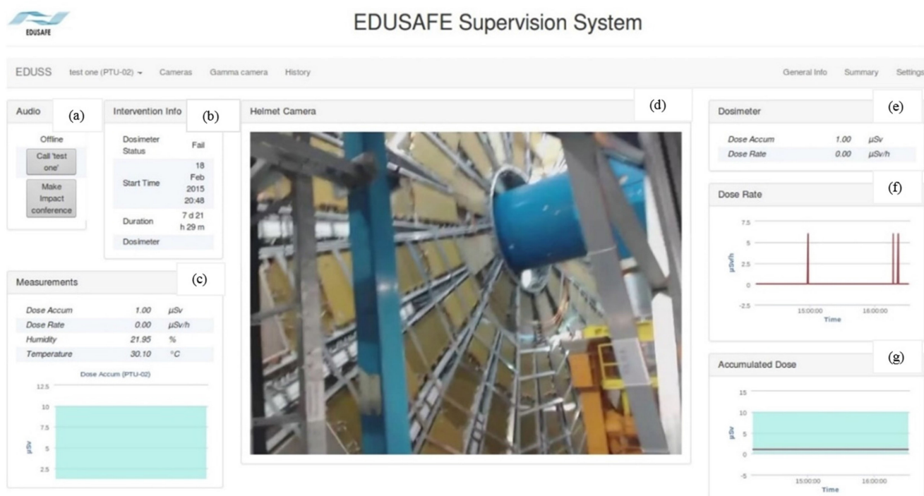
Fig. 14. Supervision user interface with measurements and video display for each user.
