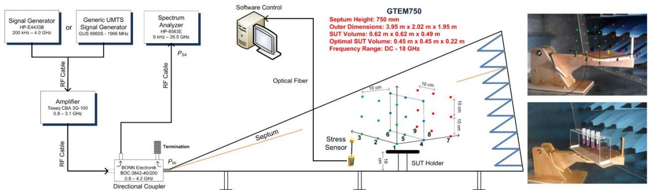
Figure 1. Field uniformity measurement setup and equipment. The photos on the right side indicate the measurement points in the GTEM cell and the location where the blood samples are positioned during the final irradiation experiment.
