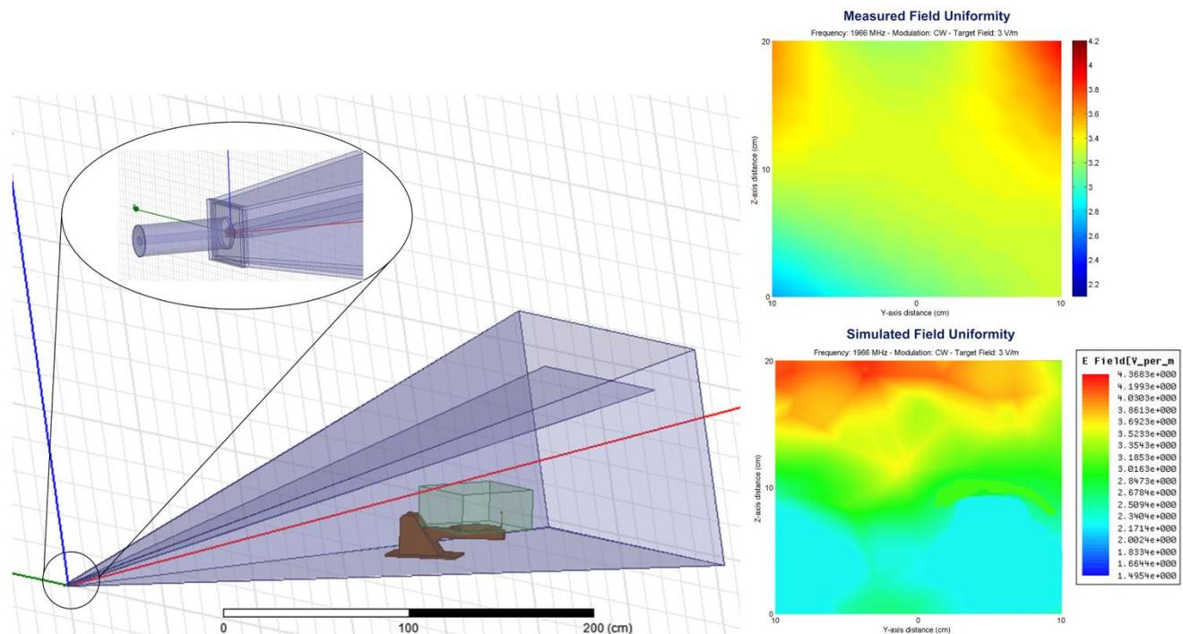
Figure 3. GTEM cell model in HFSS software. Measured and simulated electric field distributions on the central vertical plane of the considered volume (Fig. 1) for a stress level of 3 V/m and an unmodulated carrier.
