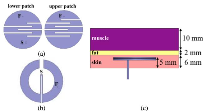
Fig. 1. Numerical simulations: (a) patch of the 204 mm<sup>3</sup> antenna, (b) patch of the 399 mm<sup>3</sup> antenna, and (c) simulation set-up.
