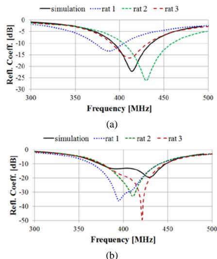
Fig. 5. Numerical and in vivo measured reflection coefficient frequency responses of the: (a) 204 mm<sup>3</sup>, and (b) 399 mm<sup>3</sup> implantable antennas.
