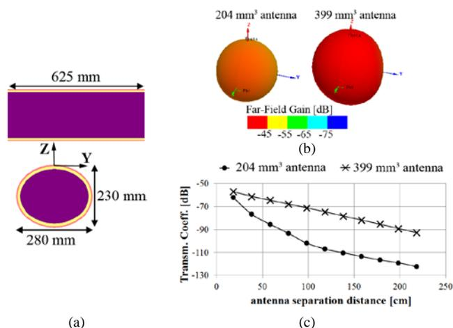
Fig. 7. Antenna performance evaluation for glucose monitoring: (a) ellipsoidal trunk model, (b) far-field gain radiation patterns, and (c) transmission coefficient considering an exterior monopole antenna.
