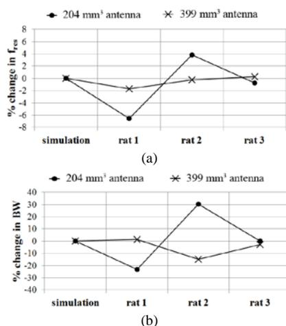
Fig. 6. Percentage changes of the following measured parameters, as compared to the corresponding numerical values: (a) center resonance frequency within the bandwidth ( $f_{res}$ ), and (b) 10 dB-bandwidth (BW).
