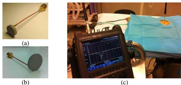
Fig. 3. In vivo measurements: (a) prototype of the 204 mm<sup>3</sup> antenna, (b) prototype of the 399 mm<sup>3</sup> antenna, and (c) experimental set-up.
