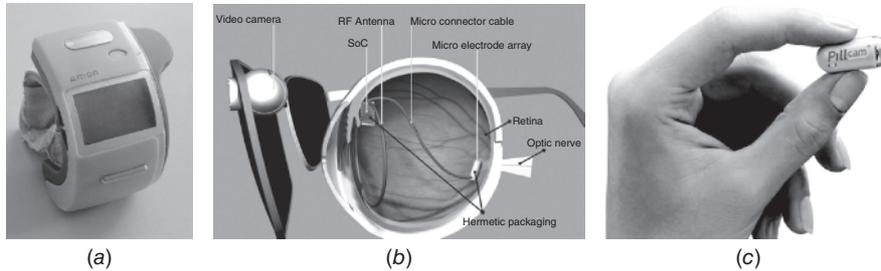
**Figure 1.1** (a) Wearable [advanced care and alert portable telemedical monitor, AMON (Anliker et al., 2004)], (b) implantable [epiretinal prosthesis (Sivaprakasam et al., 2005)], and (c) ingestible [PillCam (Mc Caffrey et al., 2008)] medical devices.
