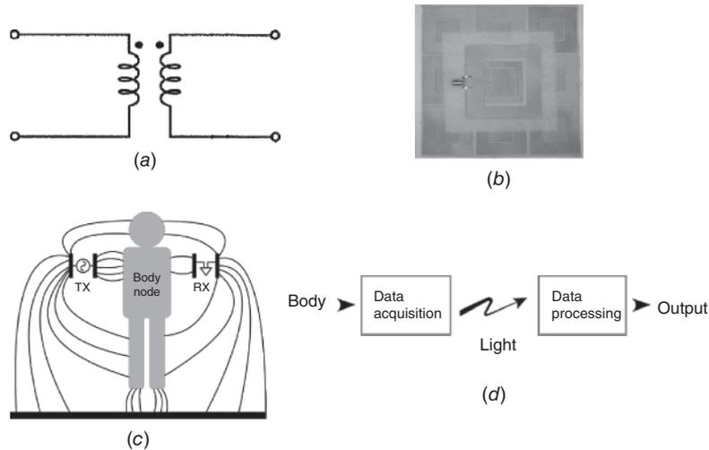
**Figure 1.3** Data transmission techniques in biomedical telemetry systems: (a) inductive coupling, (b) antennas and RF communication (dual-band wearable textile antenna (Zhu and Langley, 2009)), (c) intrabody communication (Cho et al., 2007), and (d) optical communication.
