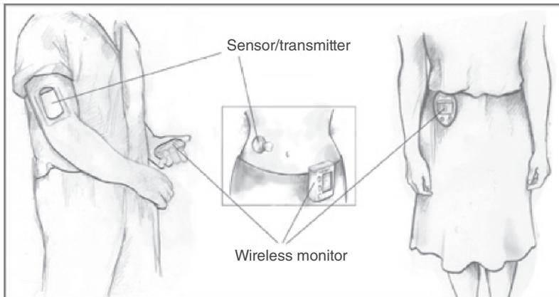
**Figure 1.7** Schematic diagram of implantable systems used for continuous glucose monitoring.
