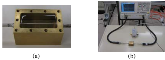
Fig. 1. MedRadio muscle-equivalent phantom: (a) coaxial container for complex permittivity measurement, and (b) experimental set-up used for measuring the phantom electrical properties.
