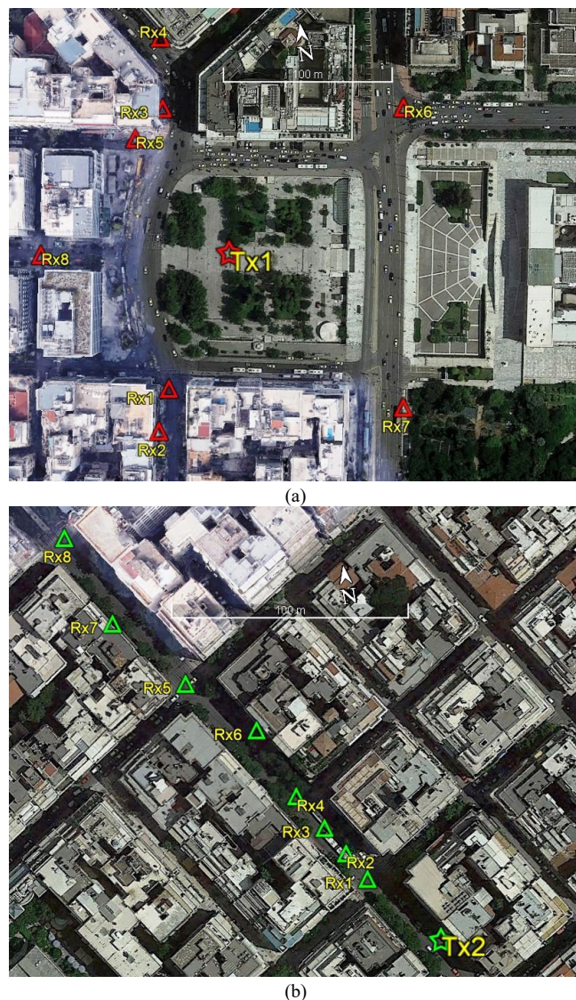
Fig. 2. Propagation study environment in parts of downtown Athens. (a) Scenario 1. (b) Scenario 2. The photos are taken from Google Earth™. The trees appearing in the area are not embedded in the digital map during the simulation procedure.
